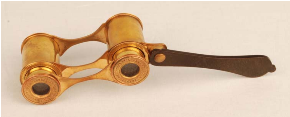
Figure 11. Lorgnette-style opera glasses with an early focusing mechanism. The left barrel is rotated to focus both telescopes, and the two eyepiece draws are attached to a third bridge. (French, early 1800s). The eyepiece inscription reads “Par Brevet de Perfectionnement,” indicating that this design is “by patent of improvement.”
