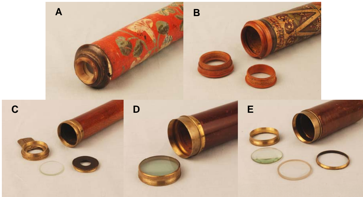
Figure 8. Objective lens mounting: (A) Lens is mounted in a turned horn cell with a horn retaining ring. The retaining ring is on the front of the lens cell (Leonardo Semitecolo, Venice, early to mid-1700s); (B) Lens is mounted in a turned wood cell with a wood retaining ring that screws into the rear of the cell (unsigned, German, early to mid-1700s); (C) Brass cell with an integral dust slide in front. The lens is held in place by a cap with a built-in aperture (unsigned, English, mid-1700s); (D) Lenses are sealed together in brass cell with a spun-over edge (Dollond, London, circa 1800); (E) Lenses are mounted in a brass cell with a retaining ring (Thomas Harris & Son, London, mid-1800s).
