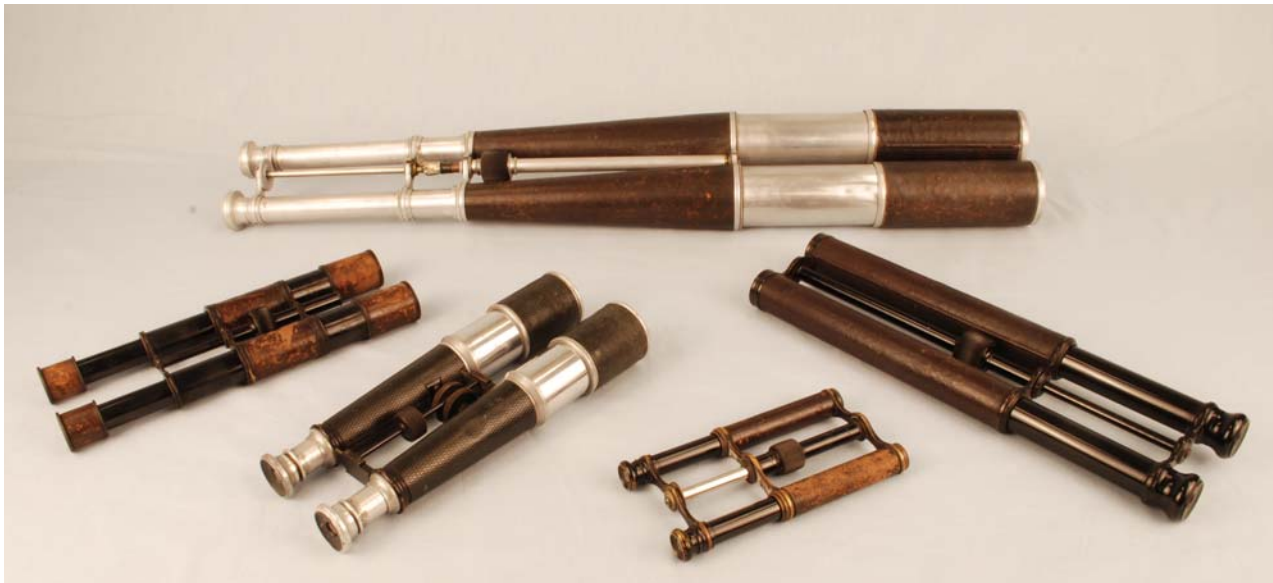
Figure 16. Various twin telescopes dating from the late 1800s. Two of the twin telescopes shown are aluminum and three are brass. The large telescope has a length of 750 mm with its sunshades extended. The magnifying powers range from about 5X to 20X.
