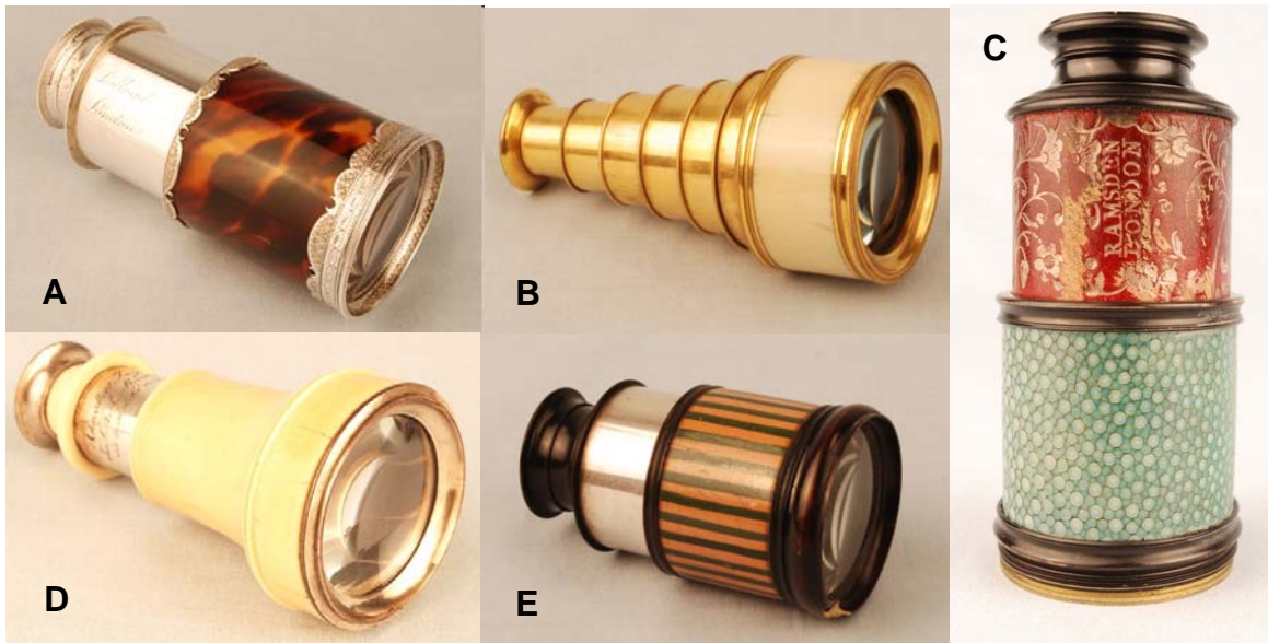
Figure 10. Galilean spyglasses: (A) Tooled silver and tortoise shell (Dollond, London); (B) Six-draw gilt brass with ivory (Dollond, London); (C) Cardboard draw with tooled leather, barrel covered with shagreen (Ramsden, London); (D) Ivory and silvered brass (Chevellier, Paris); (E) Ivory fittings with a silvered draw (Ramsden, London). All date from mid to late 1700s.
