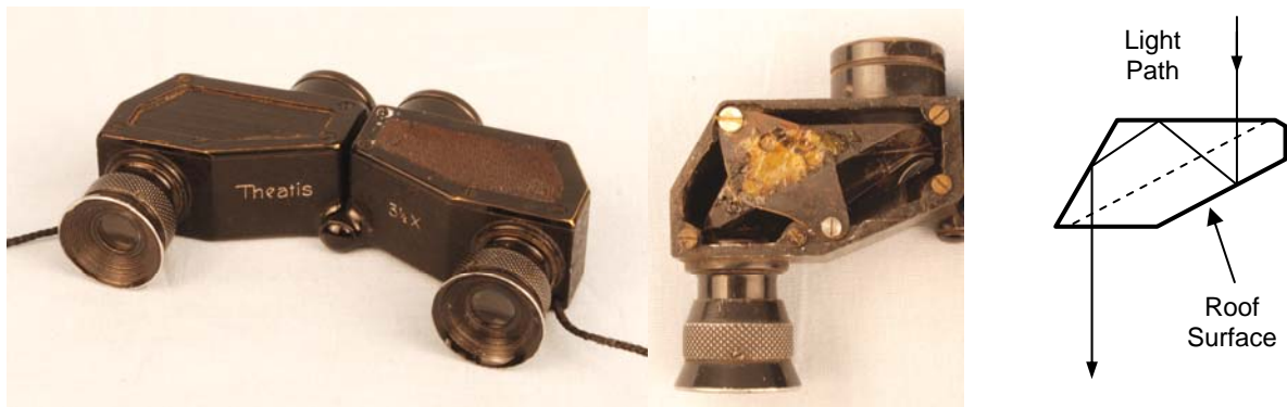
Figure 18. Leman prism binoculars (Theatis 3½X; J.D. Möller, Wedel, Germany, late 1920s). Four reflections are obtained with this compact image-erection prism.
