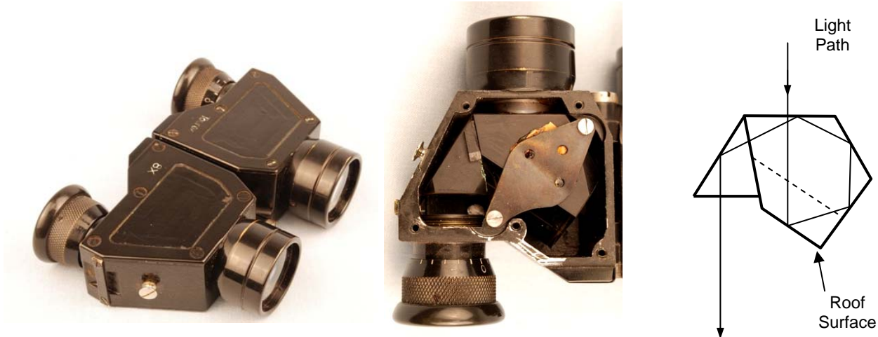
Figure 20. Möller prism binoculars (Tourox 8X; J.D. Möller, Wedel, Germany, mid-1920s). This image-erection prism system consists of two prisms that are bonded together and held in place by a spring clip. A total of six reflections are obtained.
