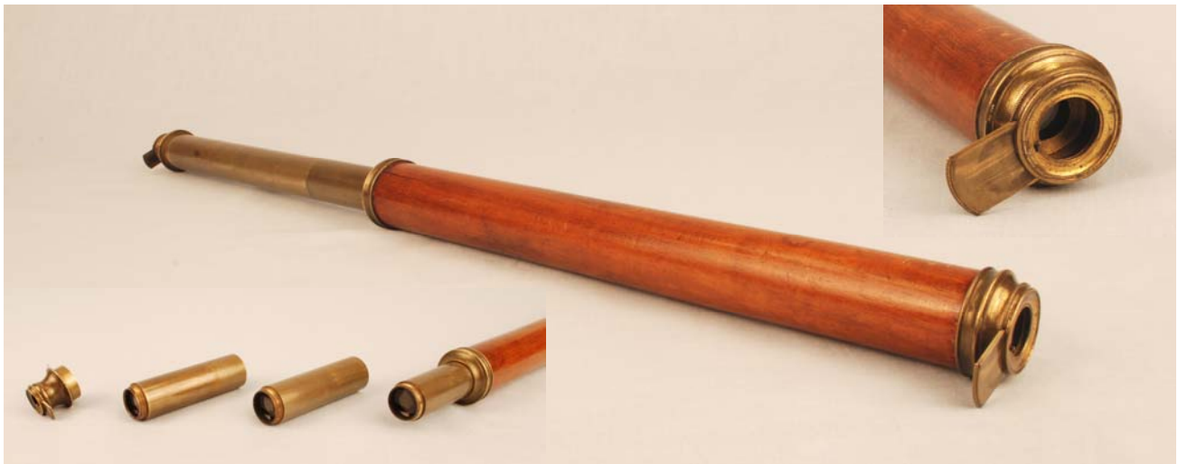
Figure 3. Single-draw pre-achromatic telescope with a wooden barrel and a Schyrle erecting system (unsigned, circa 1750, English). The telescope has an overall length of 570 mm. The objective diameter is 23 mm with a 13 mm diameter aperture. Each segment of the draw contains one of the three lenses of the Schyrle erecting system.
